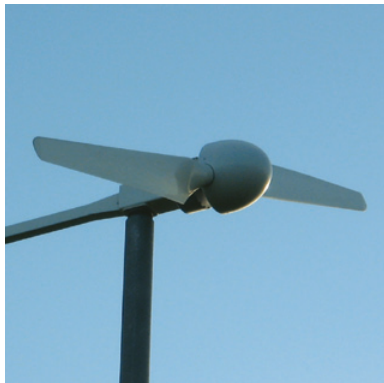
Eoltec Scirocco 6kW Wind Turbine.
